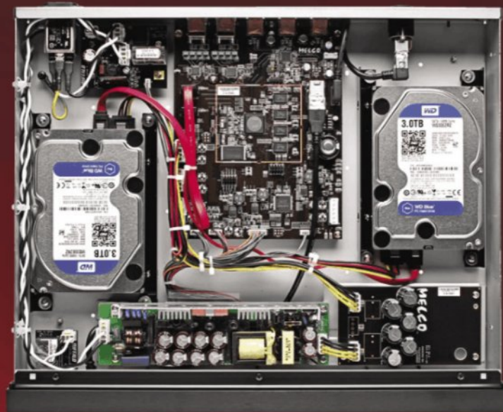
The new Melco N1A Mk2 includes two 3TB Western Digital hard disks. Other upgrades include a dedicated capacitor bank for the power supply (bottom left).
